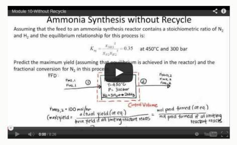
This tells us that 75% of the N2 that is fed into the reactor is going unused (i.e. wasted)! As discussed in Module 7, a major goal of chemical process engineers is to "beat equilibrium". We can do this by recycling the unused reactants back into the reactor to achieve higher overall conversion of N2 and H2.
