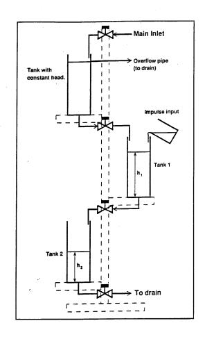
Figure 2. Configuration of Two Tanks
